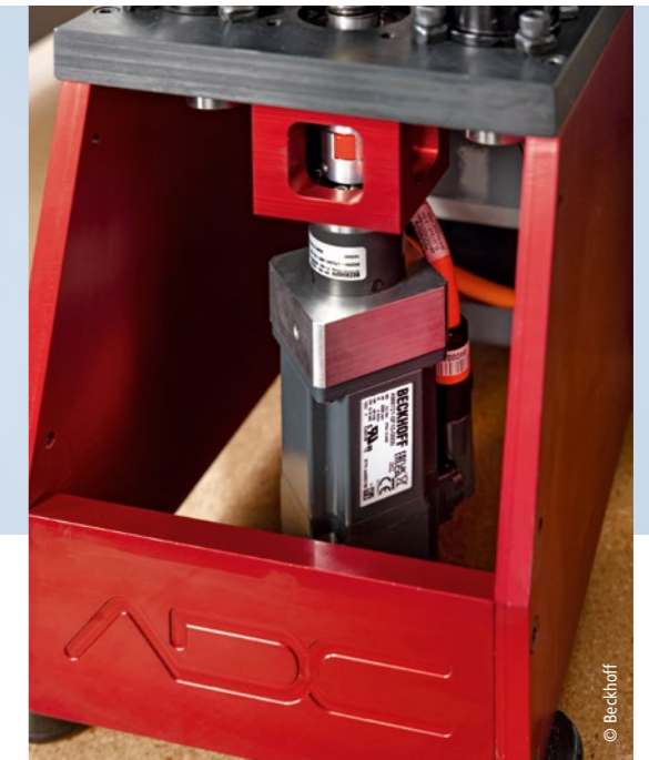
A variety of highly compact servo and stepper motor technologies (here: an AM8121 servomotor) are added advantages of the fully integrated and scalable automation platform from Beckhoff.
