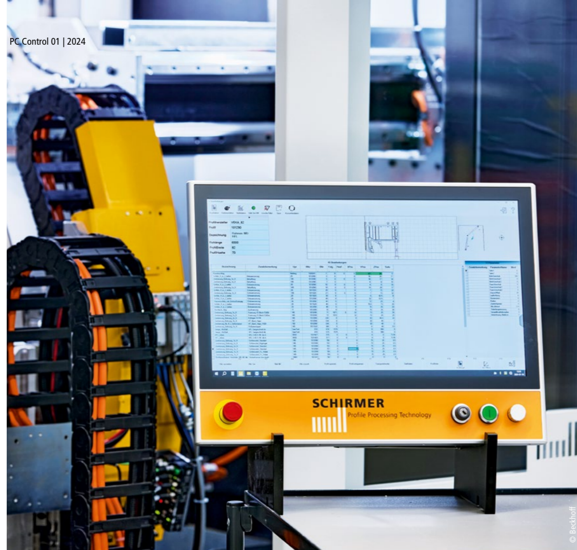
The complete machine is set up and operated via a customer-specific Beckhoff Control Panel.
