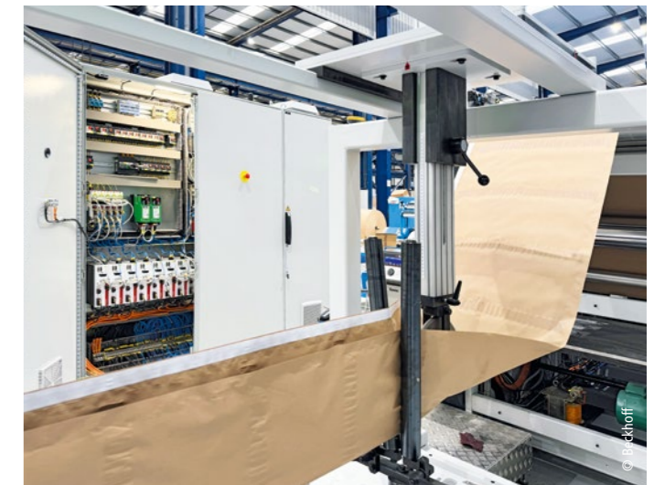
The challenge for the new implementation was the processing of multi-layer paper material into padded envelopes with high accuracy and speed.
